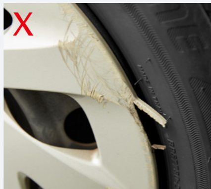
Cracked wheel trim
