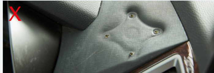
Holes in trim
