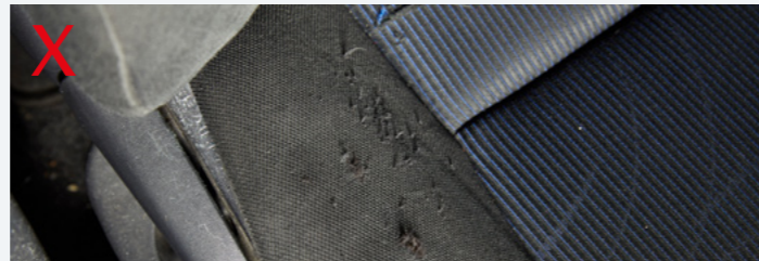
Excessive wear or rips in upholstery
