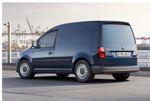
The drive systems use state-of-the-art technology, with the Caddy's new TSI petrol engine (a 1.4-litre TSI four-cylinder with a power output of 92kW / 220Nm) providing maximum efficiency and terrific performance to enable swift manoeuvrability for around-town use. Transmission options are the standard 6-speed manual or optional 7-speed DSG Automatic.
